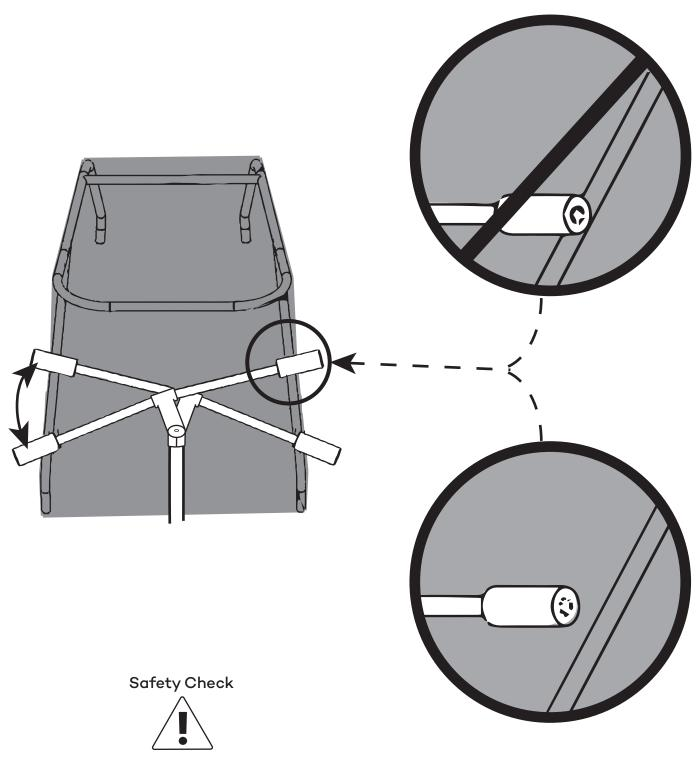
Make sure Supercargo handlebar does not interact with the Canopy frame.
